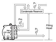
The discharge capacity is determined by the motive medium, motive medium pressure (Pm) and back pressure (P<sub>2</sub>).
